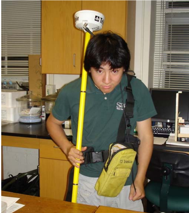
Figure 9. H. Hsu suiting up in the lab to carry out our field equipment. The Pro XR receiver and 12V batteries are in a lumbar pack clipped around his waist, the TDC1 datalogger is in the vertical front pouch, and the antenna is mounted on a yellow pole comprised of several sections for varying length and weight.
