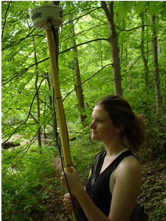
Figure 2. Plotting a vertex with the Trimble Pro XR. D. Moore holds the receiver high to aid in locating satellite reception.
